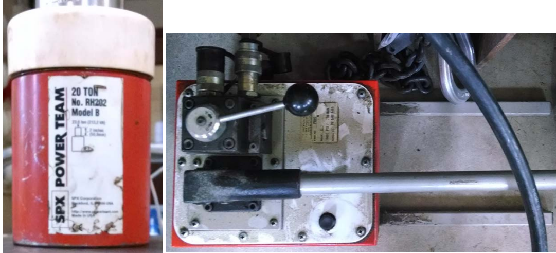
Figure 7.10 SPX Power Team RH202 Jack (Left) and SPX Power Team P460d Pump(Right)
